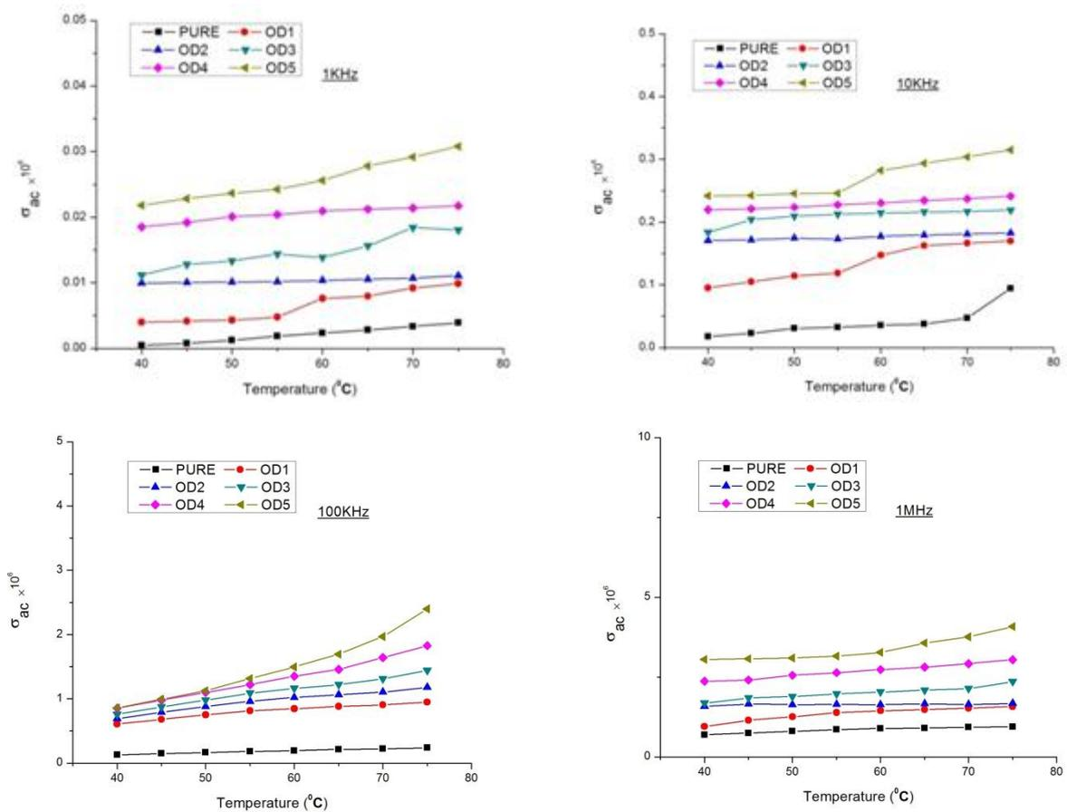
Fig4. The AC electrical conductivities ( $\times 10^{-6}$  mho/m) for pure and doped NSH crystal
