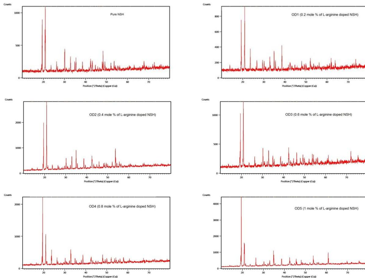
Fig2. Indexed Powder XRD pattern of pure and doped NSH crystal
