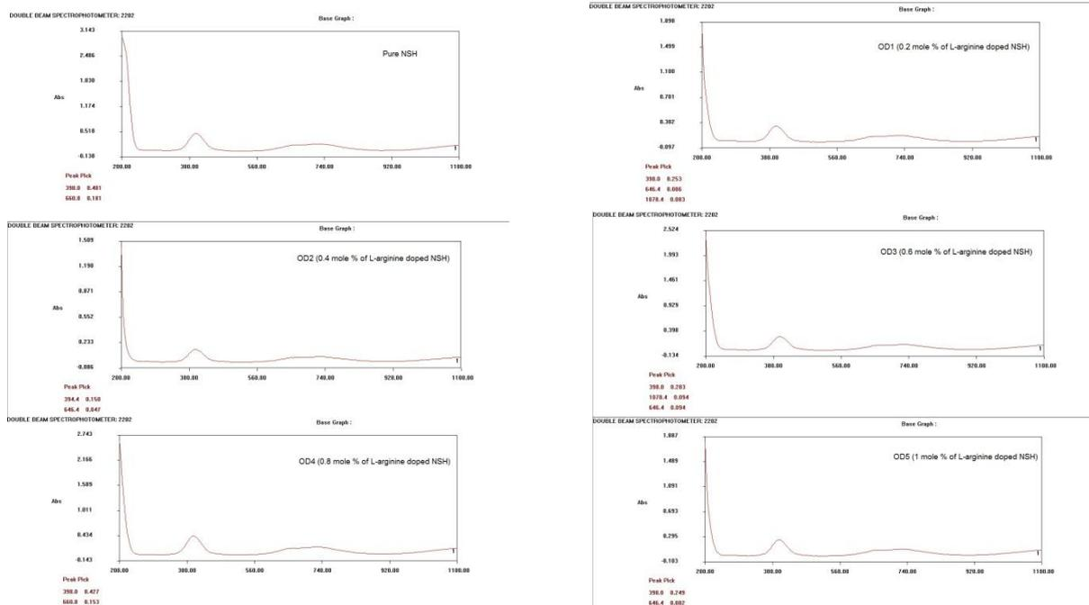
Fig6. UV-Vis-NIR spectroscopy of the pure and doped NSH crystals.
