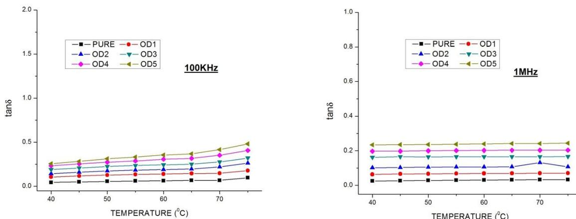
Fig5. The dielectric loss factors for pure and doped NSH crystals
